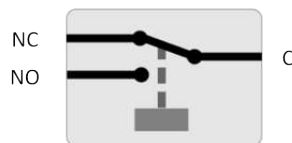
Relay configuration (not energised).
